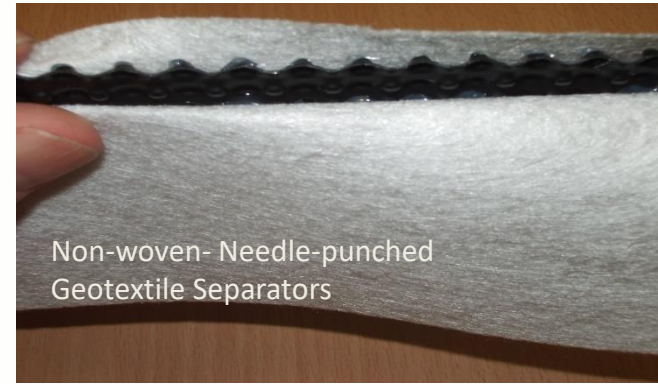
Cross Section of ABG Fildrain – double cusped 7mm thick
